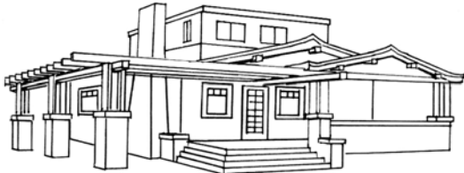
Flat roofed, unarticulated addition is not consistent with Craftsman style
