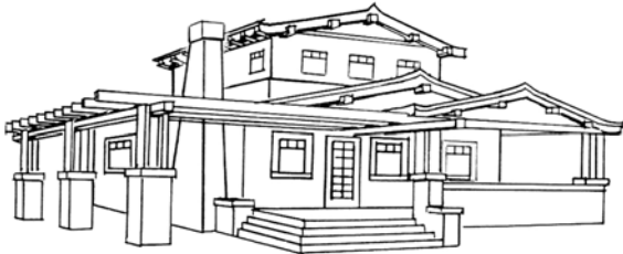
Second story addition is set back to reduce impact of added height
