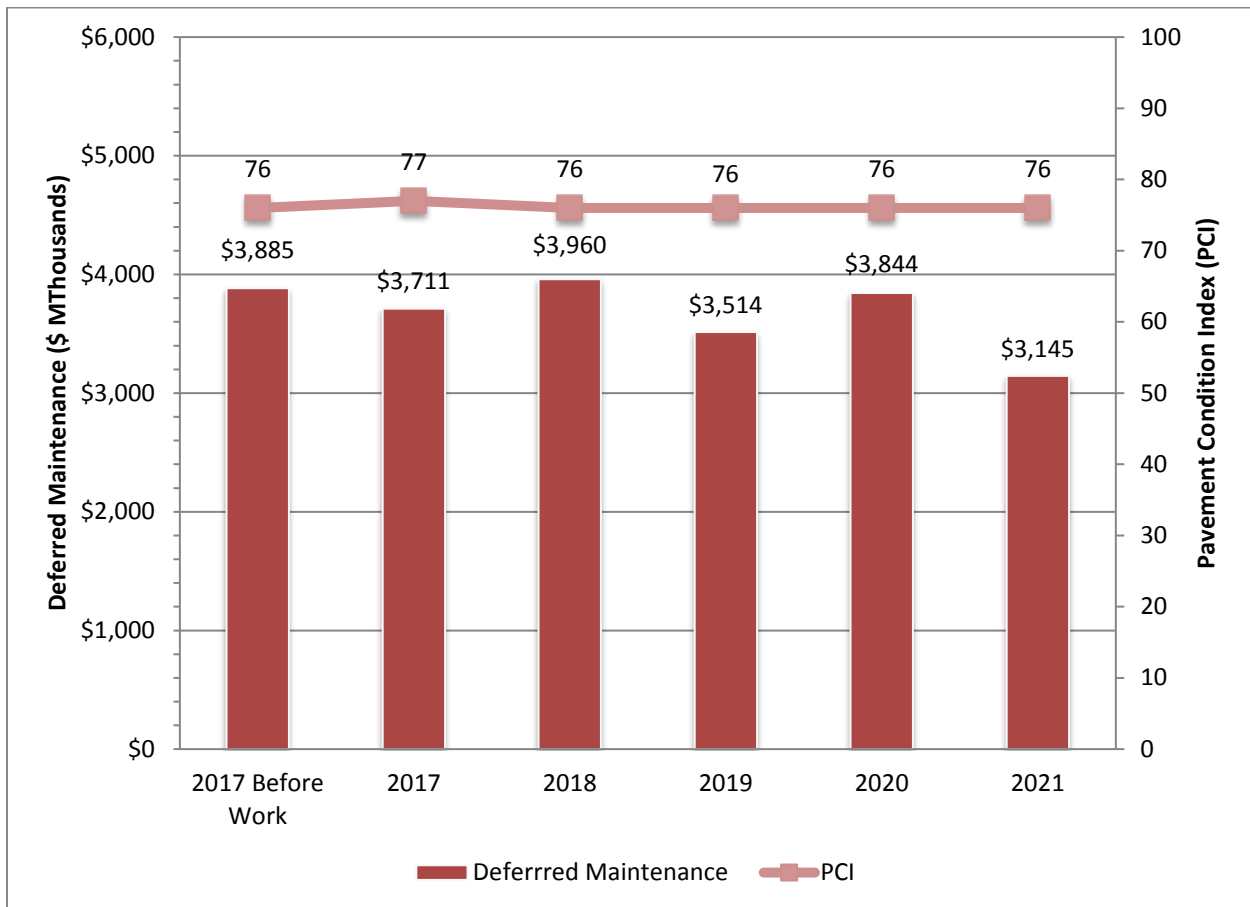
Figure 7: PCI vs Deferred Maintenance for Scenario 2
