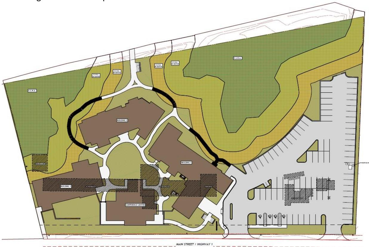
**Figure 1. Project footprint.** The proposed development and undeveloped areas. Depicted in the upper (western) portion of the drawing are lines delineating the edge of the wetland, a 30-foot and 50-foot buffer. Portions of the trail are proposed within the 50-foot buffer adjacent to the higher quality wetland and within the 30-foot buffer of the lower quality wetland.
